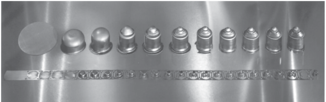
EXHIBIT 2 The Stages of a Motor Housing Stamping
